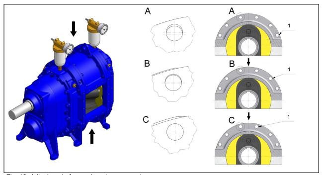
Fig. 19: Adjustment of pump housing segments
