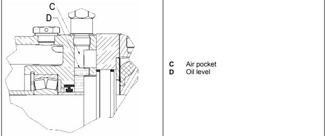
Fig. 10: Pump with pressure valve, without buffer fluid tank
