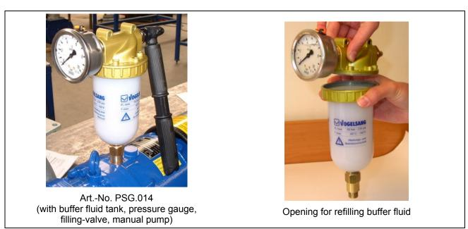
Fig. 8: Buffer chamber monitoring
