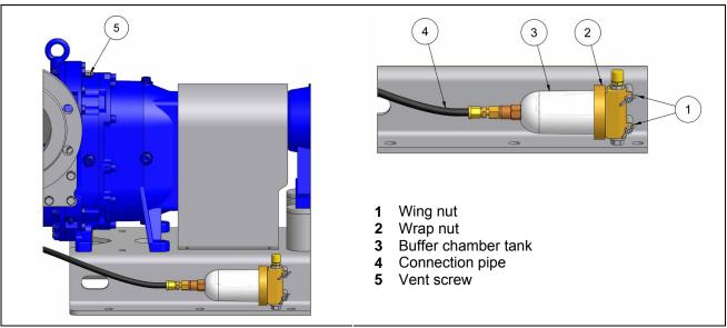
Fig. 11: Installation example - dry buffer chamber
