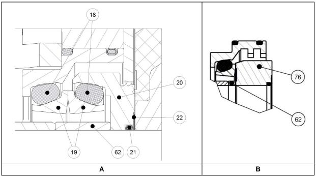
Fig. 18: Converting a mechanical seal (HD alignment) [A] to block ring mechanical seal [B]
