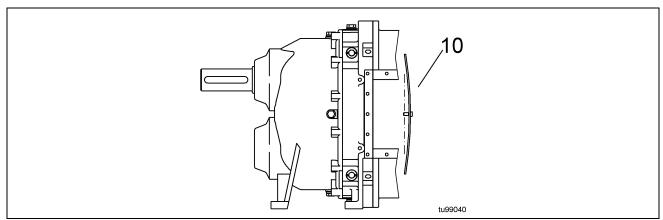
Fig. 16: Wear plate - curved design (10)
