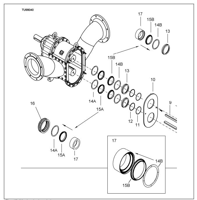
Fig. 17: Mechanical seal change
