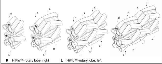
Fig. 14: HiFlo™-rotary lobe installation
