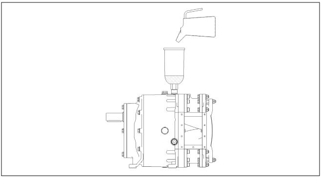
Fig. 7: Fill buffer chamber
