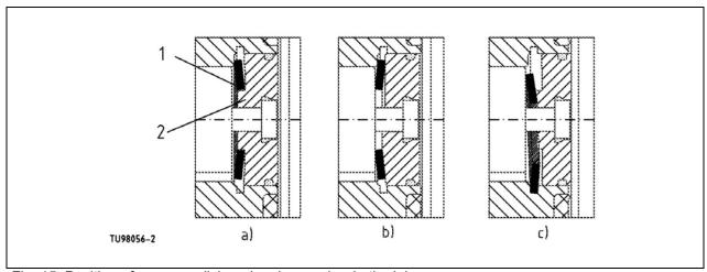
Fig. 15: Position of pressure disk and spring washer in the lobe
