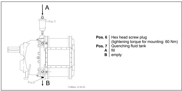
Fig. 9: Pump with quenching fluid tank, without pressure valve
